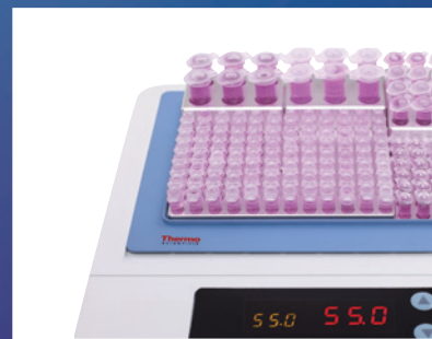
Compact Dry Bath / Block Heater pg 6
