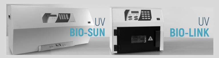
The BioSun is a complete, microprocessor controlled UV irradiation system designed for Petri dishes or micro-plates. Based on a programmable microprocessor, the system constantly monitors the UV light emission. The irradiation stops automatically when the energy received matches the programmed energy. Thanks to its advanced UV sensors, the irradiation cycles are perfectly reproducible, regardless of the intensity fluctuation of the UV source.
